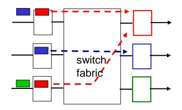
output port contention: only one red datagram can be transferred. lower red packet is blocked
